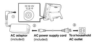
The unit is in the standby condition (the [CHARGE] indicator lights) when the AC power supply cord is connected. The primary circuit is always "live" as long as the AC adaptor is connected to an electrical outlet.
